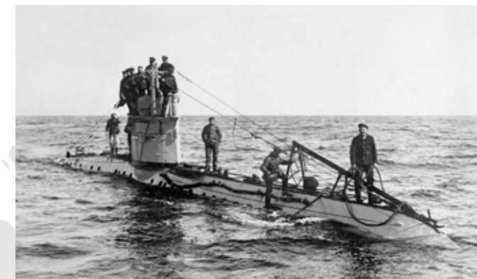
Above, Dangerous waters : The crew of a German UC-1 class submarine on deck. Introduced in 1915, such craft were employed mainly on mine-laying duties and contributed to the sinking of 1,845,000 tonnes of Allied and neutral shipping between February and April 1917. Credit: IWM (Q 20220)
